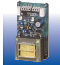
Linear CIFR modules Size : W 100 x H 170 x D 85 mm
