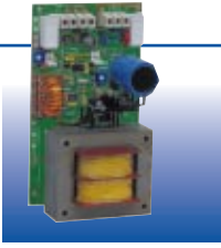
Switch mode CIFR modules Size : W 100 x H 170 x D 80 mm
