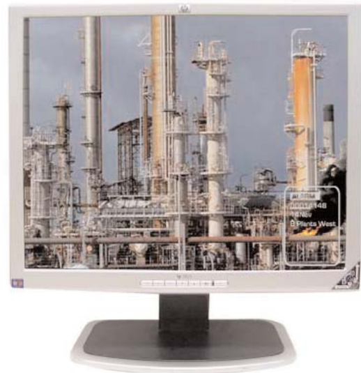
FLAMEVision alarm superimposed on the CCTV image (Illustration only)
